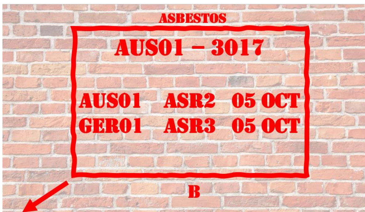
Figure 15: Australia 01 have completed an ASR 2 Sector Assessment at the specific Worksite C-1c.
