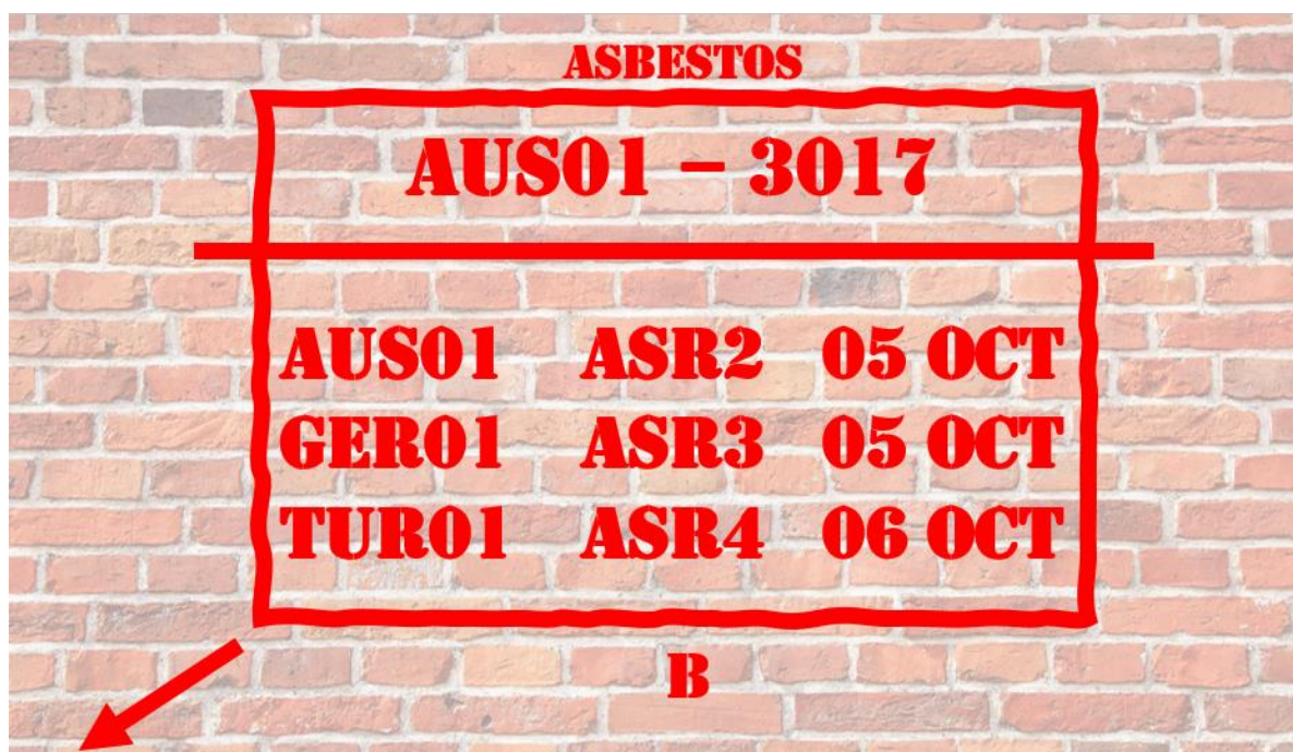
Figure17: Türkiye 01 having completed ASR 4 Full SAR on the AUS01-3017 worksite, having determined no further work is required on this worksite.
